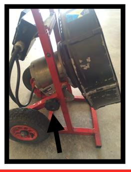
Note the side adjustment knob, this allows the blade housing to be moved up or down to enhance flow and better encapsulate the desired in-flow opening
