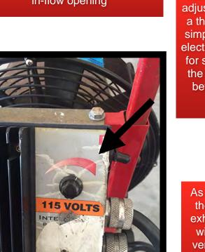
Many fans have an adjustment either via a throttle for gas or simple turn knob on electric, this is allows for speed control of the fan to allow for better ventilation control
