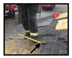
The blade does not provide a good cutting edge for roof ventilation, it has a tendency to bind and stick in the roof materials. If it does get stuck, place your foot under the axe shaft and use it as a fulcrum to release the axe.
