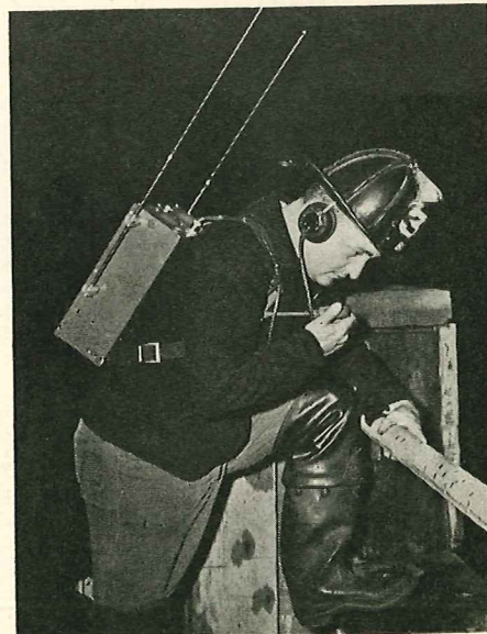
Type of portable, "back-pack" two-way radio designed by two young radio experts of the New York Fire Department, Arthur H. Meyerson and Samuel Hamatuk, which was demonstrated to representatives of the British Central Scientific Agency, and the National Office of Civilian Defense during the critical days of the war. Picture shows fireman Meyerson talking with a co-fireman on the ground from the roof of a New York skyscraper.
