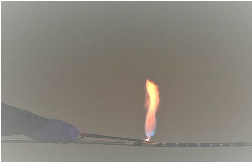
Figure 17: Approximate flame that would have come from the CSST perforation.
