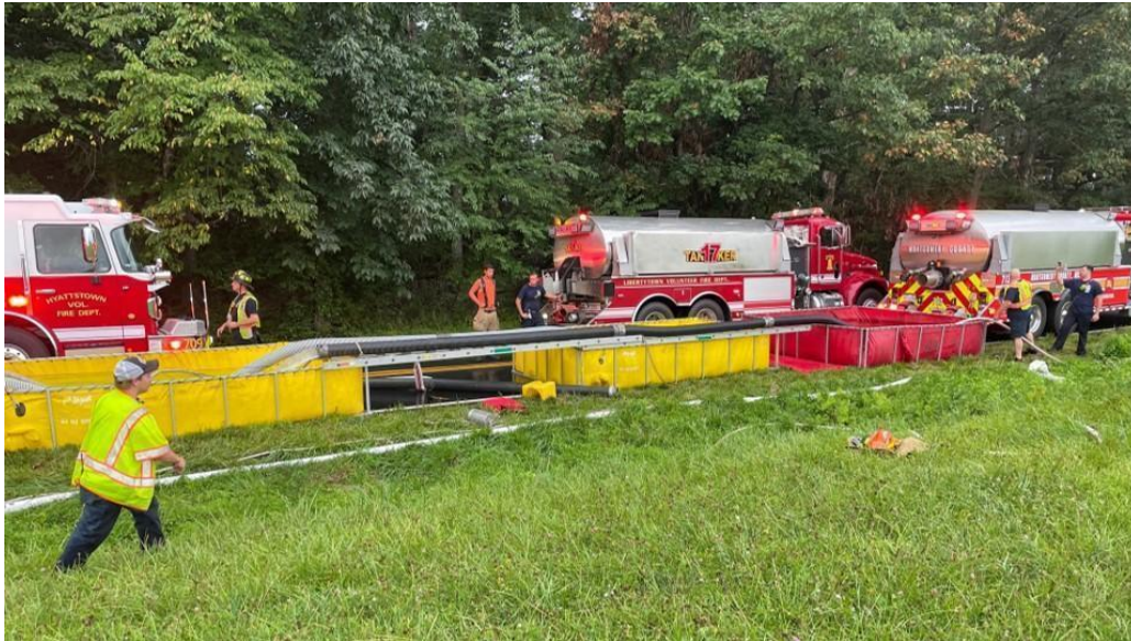
Figure 28: Water transfer between dump tanks.
