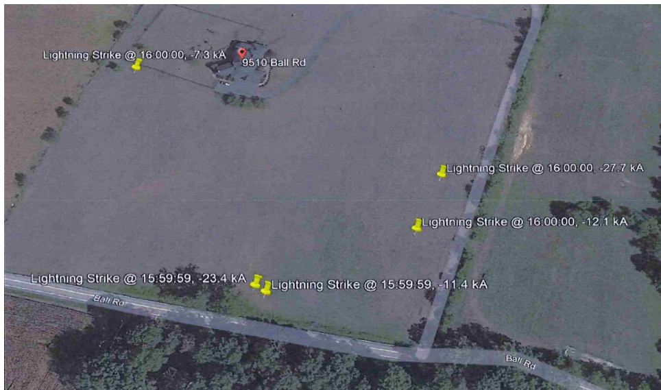
Figure 6: Visual representation of the lightning strikes in and around the area of the Ball Road structure.
