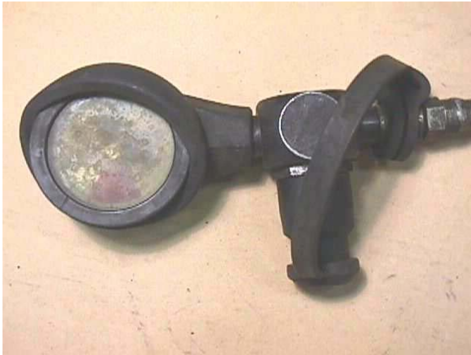
Figure 12 – Charring of Gauge Hose Jacket
